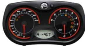
**AMBIENT AIR & ENGINE TEMPERATURE MODULE**
