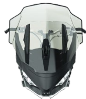
ADJUSTABLE WINDSHIELD HIGH TO EXTRA HIGH 860201782 59 cm - 69 cm. RADIEN / RADIEN-X
